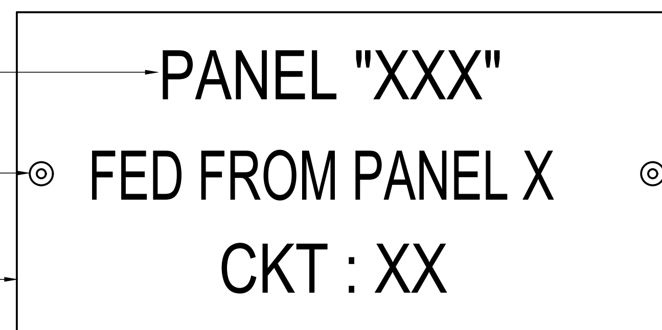
08 EQUIPMENT IDENTIFICATION LABEL DETAIL
