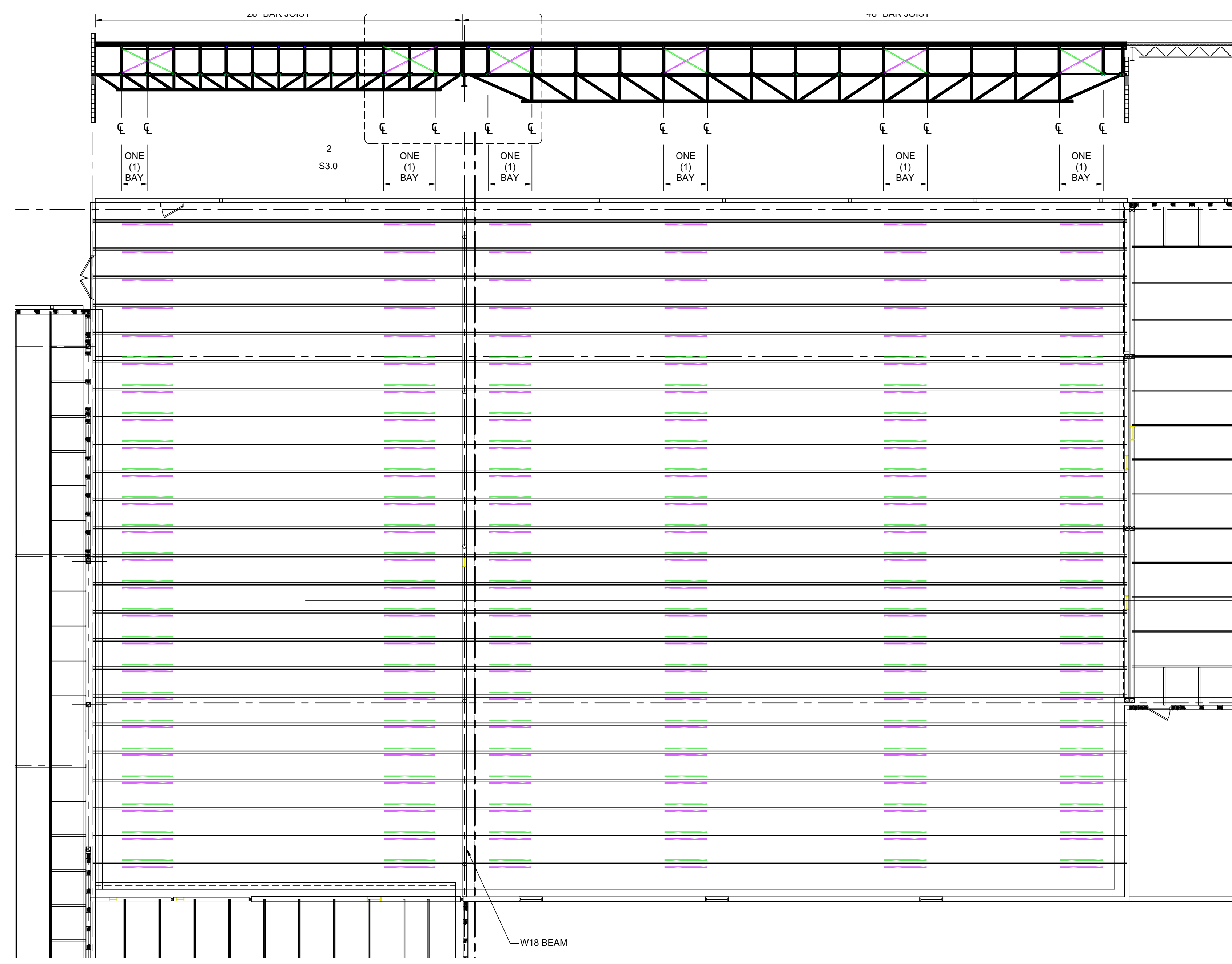
1 BRACING PLAN ROOF AREA "B" AND "C" 1" = 10' - 0"
