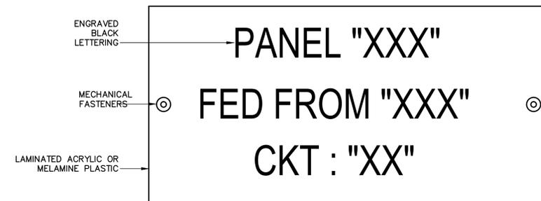
NOTE: ATTACH NAMEPLATES TO ALL ELECTRICAL GEAR AS NOTED ON SECTION 260553.
