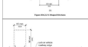
Figure 809.2.2 Dimensions of Bus Boarding and Alighting Areas
